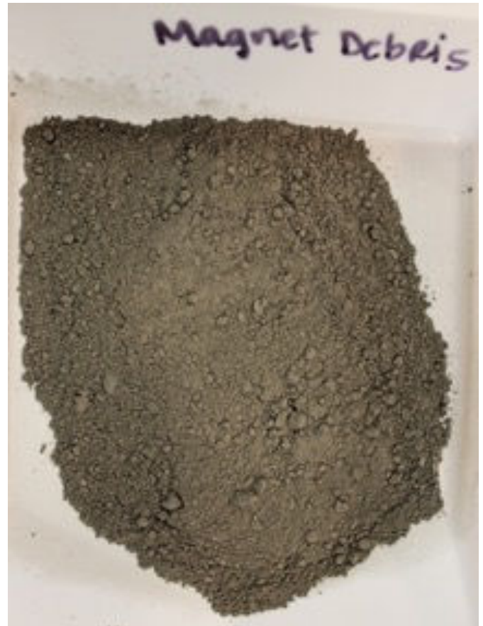
Figure 7: Sample of magnet box debris
