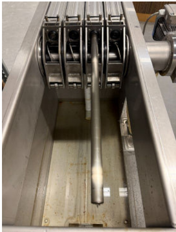
Highly efficient titanium magnet rods
