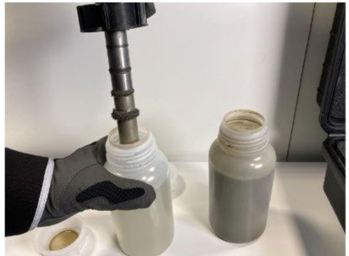
FIGURE 5: WASHING OFF DRILLING FLUID RESIDUE FOR DETERMINATION OF MAGNETIC CONTENT IN DRILLING FLUIDS.
